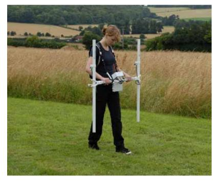
The Bartington gradiometer needs little introduction and has over recent years been the magnetometer of choice in Archaeology. Allied Associates have several instruments in their rental pool to support long and short duration hire.
