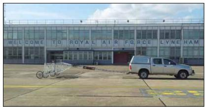
Figure 1: Towed magnetometer array at RAF Lyneham, surveying as part of the transition program.
