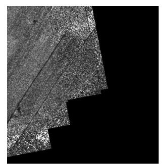
Fig. 2: Improvement of the signal/noiseratio by stacking nine distinct SAR images. The effect can be shown very clearly at the edge of the composite image.
