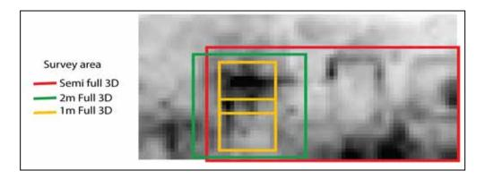
Figure 3. Comparative plot of all the electrical imaging surveys undertaken imposed on the original earth resistance grayscale
