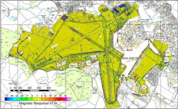
Figure 4: Magnetometer results from RAF Lyneham, acquired using a towed magnetometer array using 0.5m spaced forester gradiometer probes under RTK GPS control.
