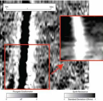
Fig. 2 Fluxgate gradiometer survey over the ditch at Cherry Copse with associated earth resistance survey area outlined in red
