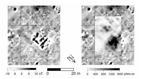
Fig. 3. Magnetic map (left) and resistivity map superimposed on the magnetic map (right). Linear features of low magnetic values in the upper part of the map can indicate both mud and stone structures. The resistivity survey showed that the structures are characterized by a high.
