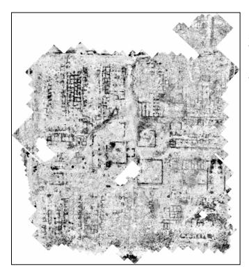
Fig. 3: GPR depth slice between 20 and 30 cm depth. GSSI SIR-3000 with 400 MHz antenna; Sensor&Software Noggin with 500 MHz antenna; PulseEKKO 1000 with 900 MHz antenna.
