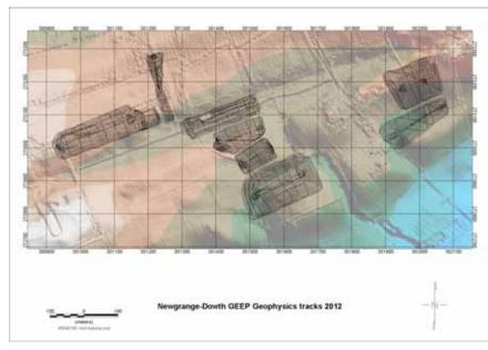
Fig 4: GEEP survey coverage superimposed on LiDAR data. Site E Is located at 301400E, 273000N.Lidar data courtesy Meath County Council and the Discovery Programme. (image : Ian Hill) The GEEP results and a comparative study of GEEP collected data with traditional hand-carried magnetic gradiometry, earth resistance and magnetic susceptibility survey will be presented.
