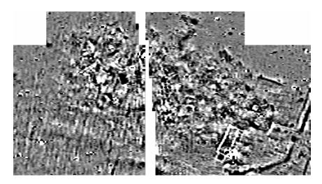
Figure 1. Fluxgate gradiometry results from a multi-period intensively occupied settlement undiscovered by other methods adjacent to the site of a 'mirror' burial. Note towards the bottom right of the plot the clear negative response of the walls of a Roman building, one wing of a range detailed further by earth resistivity. Interpolated 0.125x1.0m reading intervals. Grid size20x20m. Survey area 160x100m. Black positive & white negative. Clipped at -5 to +5 nT
