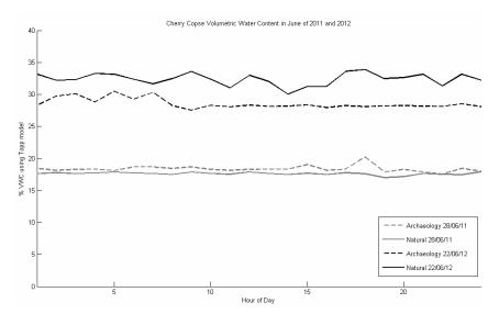
Fig.4 Calculated volumetric moisture content throughout each survey day from two TDR probes placed at depths between 20-30 cm within the ditch-fill and the 'natural' at Cherry Copse
