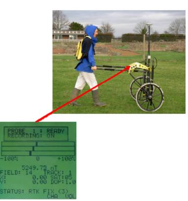
compensate disturbing influences from large anomalies at large distance to probe. Small magnetic anomalies close to the probe/surface will be displayed with high special resolution and high contrast.
