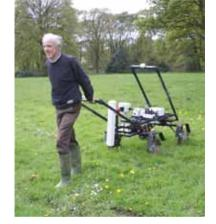
output is available for the ADVANCED model for connecting to external wheeled systems. There is also a GPS logging option for the ADVANCED model that records GPS position with each reading (user supplied GPS unit) and provides real time monitoring / feedback of GPS signal Quality and DOP.
