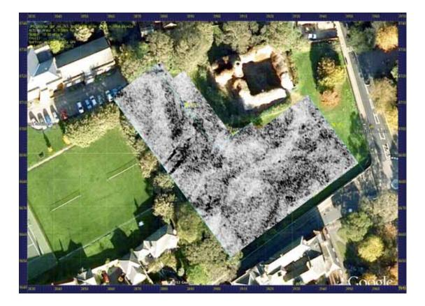
Figure 2. GPR timeslice (Mala 500 MHz instrument) at 34 ns (≈ 1.7m).
