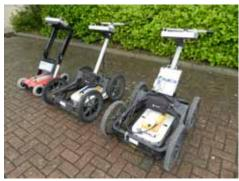
**Towed Instrument system**; Unique to Geomatrix is the Geophysical Equipment Exploration Platform (GEEP). GEEP offers the ability to record multiple data sets from complimentary instrumentation on a single towed platform. GEEP permits large areas to be surveyed in great detail and at high speeds whilst maintaining high data quality.
