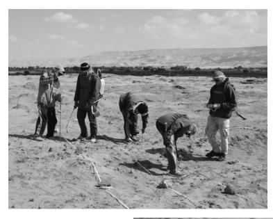
Fig. 4. Resistivity survey. On the left a team making and watering holes in the ground.
