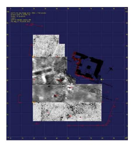
**Figure 3**. **Ground resistance.** White indicates higher resistance than average, black lower. The survey grid is based on GSB's from 1997. Grid axes in metres, arbitrary origin. Numbered survey points locate site features.
