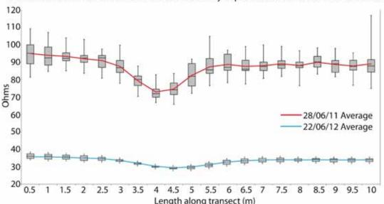
Earth resistance measurements over the ditch at Cherry Copse between June 2011 and June 2012
