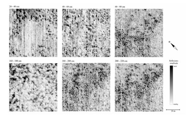
Fig. 4. Map of a complementary ground penetrating radar survey supporting the results of previous magnetometer data measurements as a detailed case study in 2012. Depth slices 20 - 80 cm and 160 - 220 cm. GSSI SIR-300 with 400 MHz-antenna, sample interval 0.02 x 0.25 m, 40 m grid.
