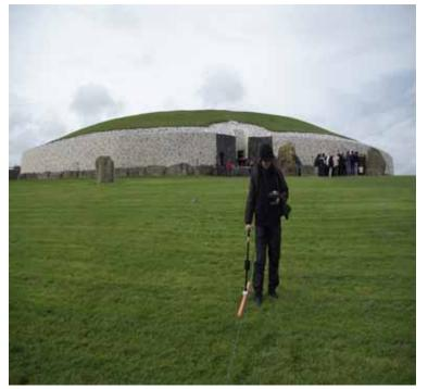
The MiniExplorer is designed for agriculture, forestry or archaeology applications providing detailed results at depths up to 1.8m. The instrument allows simultaneous measurement with 3 depth ranges (0.5, 1, & 1.8M) making this an ideal complement to the traditional surveying techniques. Lightweight, fast and GPS compatible this new product will offer increased knowledge of the subsurface. Sales are rental of the Mimi Explorer are available.
