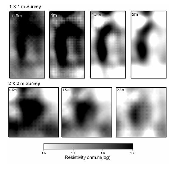
Figure 4. Data collected from a full-3D survey over the rectangular building at both 1m gridded probe separation, and at 2m gridded probe separation.
