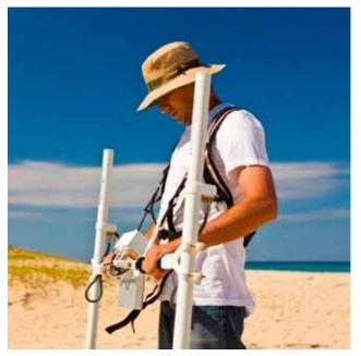
The Grad601 gradiometer is an ideal instrument for magnetometry surveys in archaeology. Since its introduction in 2004 it has rapidly gained an enviable reputation for its ease of use, automatic set-up and excellent stability. With a 1m vertical sensor separation and a high resolution of 0.01nT, recorded data is of a very high quality, whilst fluxgate technology ensures it is one of the lightest instruments available. The sensors are also available individually for cart assembly.
