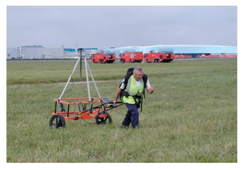
**Figure 3.** Ian Wilkins of GSB Prospection Ltd using an EM-61 with dGPS. Photograph courtesy of GSB.
