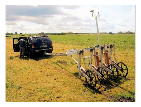
**Figure 5**. Squid system developed by Schultze and colleagues ate the Institute for Physical High Technology, Jena (Germany).
