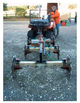
In addition to data collection at great speed the SQUID technology allows very accurate measurements, easily outperforming other magnetic devices (Schultze et al 2005). The latest incarnation of the French mechanised resistivity system also has its roots in a non-archaeological application (viniculture) (**Figure 6**). Again, this is directed by real time GPS and can measure three depths of resistivity simultaneously (Dabas and Favard, 2004).
