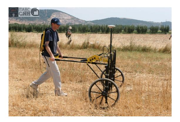
**Figure 4.** The Foerster FEREX system in operation at the University of Sienna Summer School at Grossetto, 2006. Photograph courtesy of the organisers of the school.
