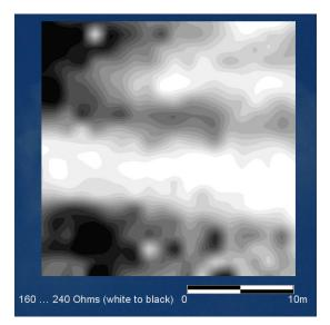
Twin-probe pseudosections were undertaken across it showing clearly the variation of resistivity, and hence moisture content, in the different layers of the fill.
