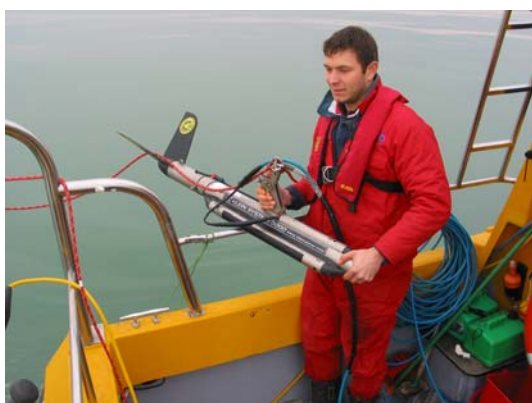
Figure 1. Klein 3000 sidescan sonar towfish being deployed from vessel.
