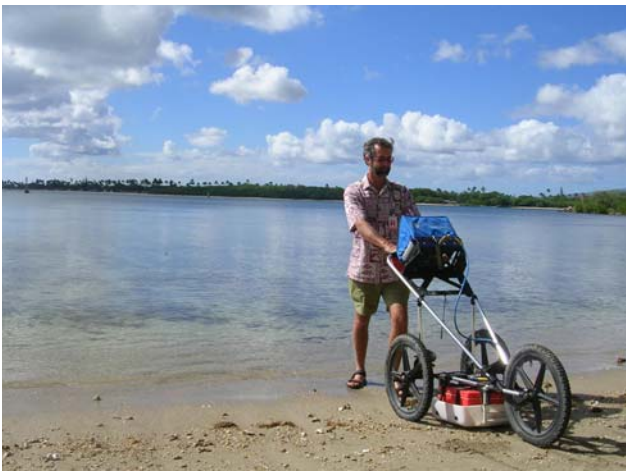
Collecting GPR at the ocean's edge in Hawaii with the SIR-3000 system and a 400 MHz antenna
