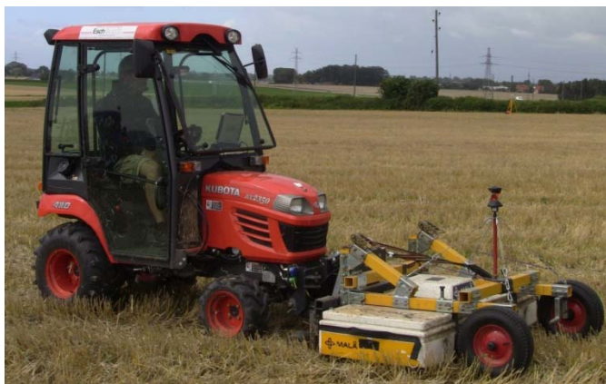
Motorized GPR survey at Uppåkra in southern Sweden with the 16 channel 400 MHz MALÅ Imaging Array (8 cm channel spacing) using a robotic total-station for positioning.
