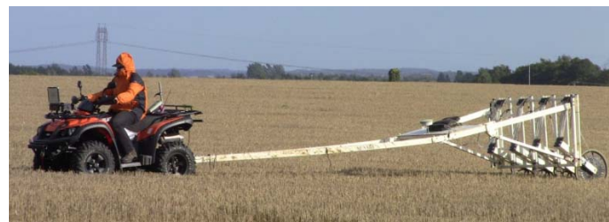
Motorized magnetometer system carrying five Foerster gradiometer probes with 50 cm spacing.
