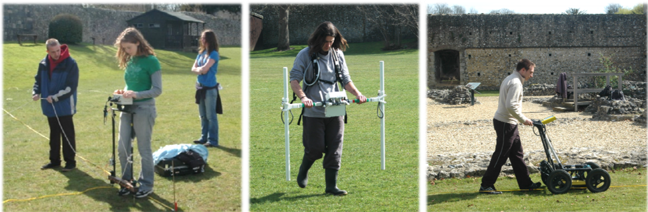
Figures 1-3: 2009 survey undertaken at Wolvesey Palace with 1: Earth Resistance, 2: Magnetometry 3: GPR
