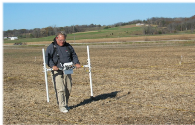
Figure 2: Magnetic survey with a Bartington Grad 601-2
