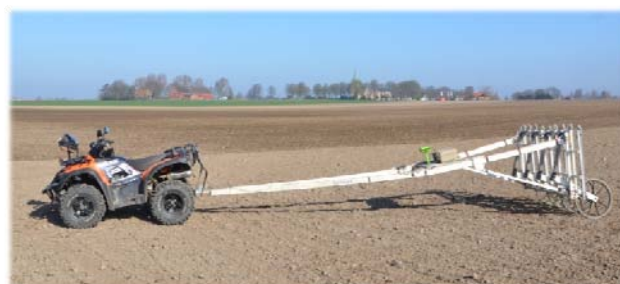
Figure 2: Motorized magnetic survey with 10-channel Foerster gradiometer array mounted with 25 cm probe spacing on a nonmagnetic cart in April 2011. The RTK-GPS antenna for data positioning is visible on the cart. In the background Uppåkra church can be seen.
