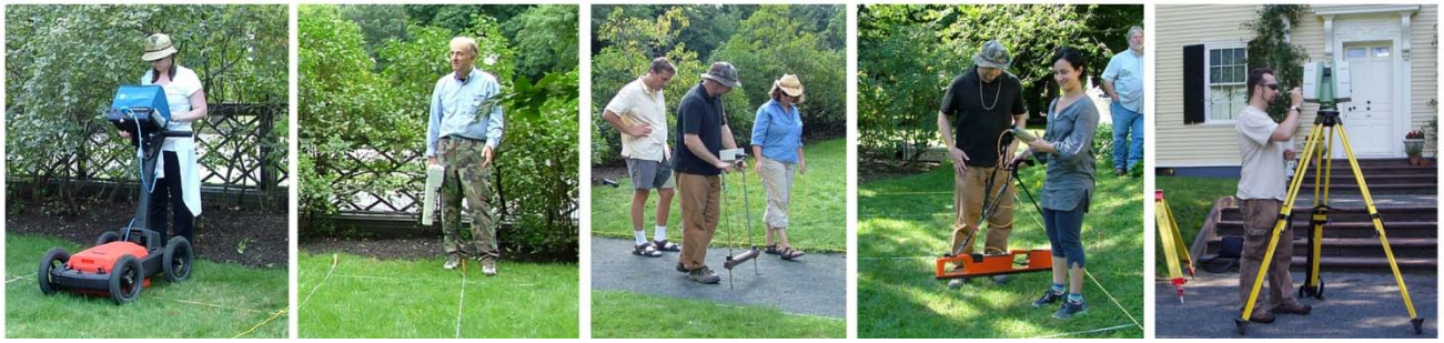
Figure 2 Survey techniques for the ASTDA workshop included: the SIR3000 GPR with a 400 MHz antenna, the FM256 Fluxgate Gradiometer (with instructor Ken Kvamme), the TR/CIA Resistance Meter (with instructor Bryan Haley), the EM38B conductivity meter, and a Leica ScanStation C10 3D laser scanner (with instructor Steve Wilkes).
