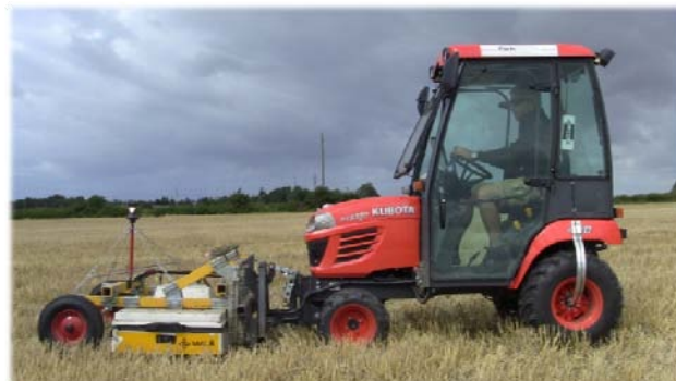
Figure 1: GPR measurements with the 16 channel 400 MHz MALÅ Imaging Radar Array (MIRA) with 8 cm channel spacing using a robotic total-station together with a prism for automated data positioning.
