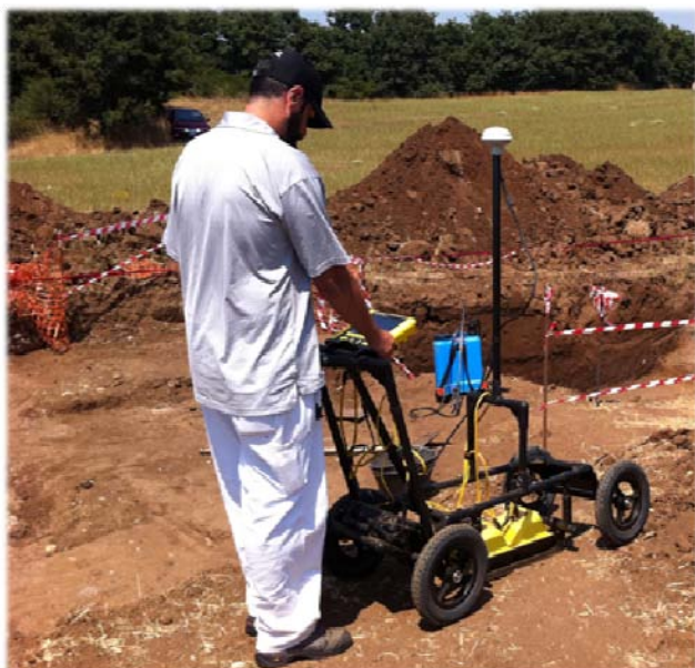
Figure 1: The GPR system involved in the Colle Rotondo survey
