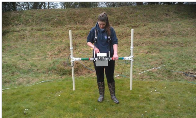
Figure 2 Magnetometer survey being carried out by one of the Southampton students, using a Bartington Instruments Grad 601 fluxgate gradiometer (photo: K. Strutt)
