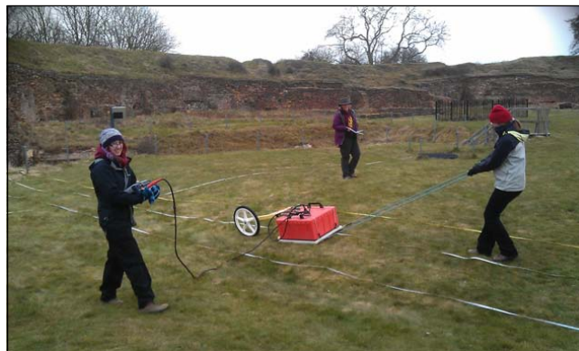
Figure 3 GPR survey being undertaken in the Old House using a GSSI 200MHz antenna with SIR-3000 (photo: K. Strutt)
