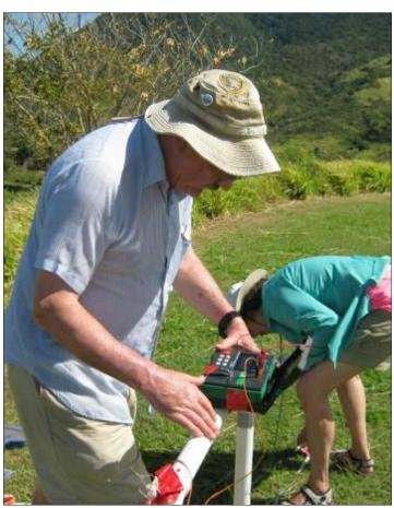
Figure 1 Photo of the author operating the DY4300 resistivity meter mounted on the PVC pipe frame.
