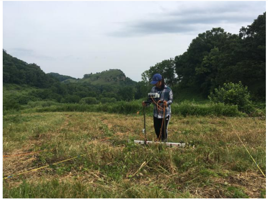
Figure 2: Linh Luong collecting earth resistance data.
