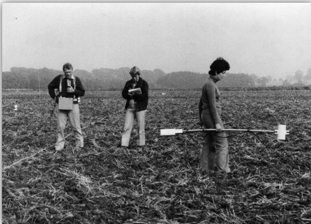
Figure 8: Left to right: Fro Rainey, Beth Ralph and Marina Someone holding the sensor. Note that this was in the days when Fro was calling out each reading, written down by Beth and plotted out - usually by me - in the evening (Rog Palmer about the 1970' survey in Kingscote, Gloucestershire).
