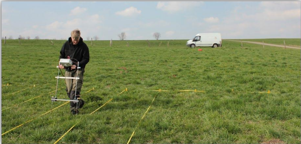
Figure 7: Benny Rieger performing a test survey over a Roman cellar with his home-made resistivity meter. The first survey ended with really bad results, caused by some pcb failures. But after everything had been modified he decided to give it another try. Finally there were really good result for such a unit (Picture and description from Benny Rieger).
