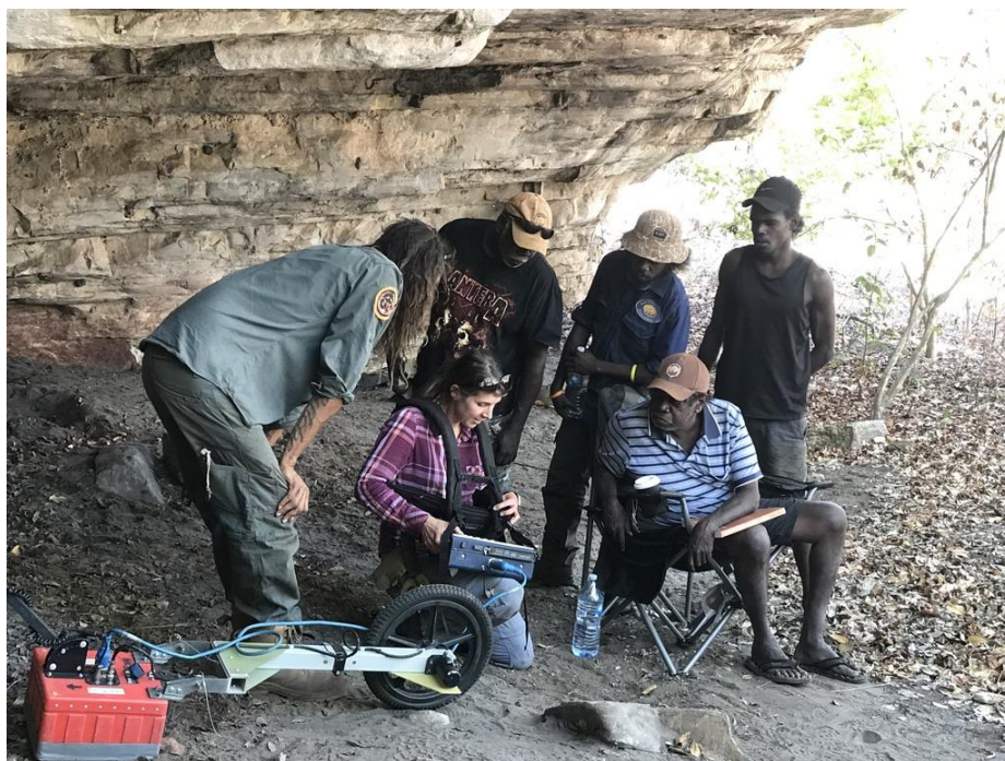
Figure 2: Dr Kelsey Lowe showing the Njanjma Rangers how GPR works.
