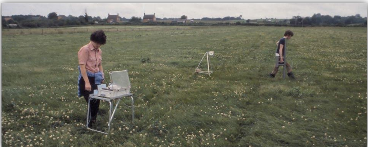
Figure 12: Andrew David back in 1980 surveying with a Littlemore 1m fluxgate gradiometer with Beverly Thomas managing the x-y plotter (content provided by Paul Cheetham).
