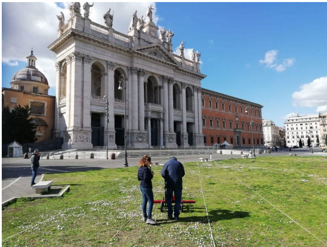
Figure 2: The CNR team surveying in front of St. John Lateran Basilica using a 70 MHz monostatic antenna, March 2020. Photo Ian Haynes.
