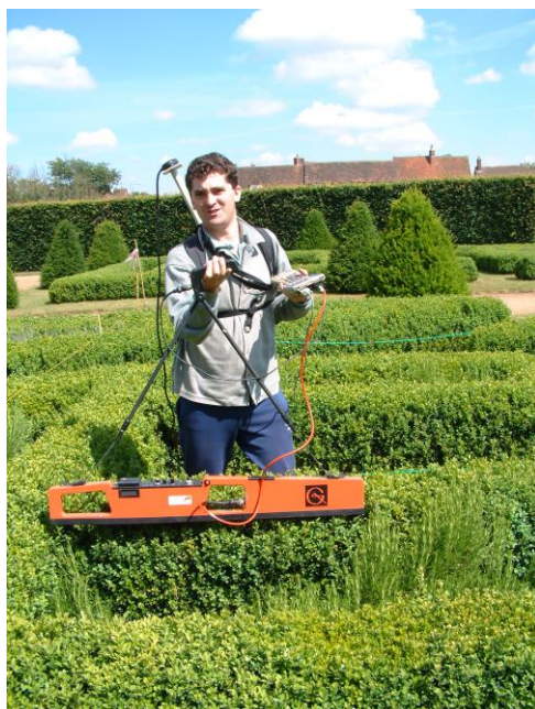
Figure 4: In-phase EM measurements proved useful for detecting former paths within the formal garden laid out in the 1970s at Kenilworth castle. Magnetically enhanced material that was used to form the original cinder paths has produced positive responses shown in white on the plot.
