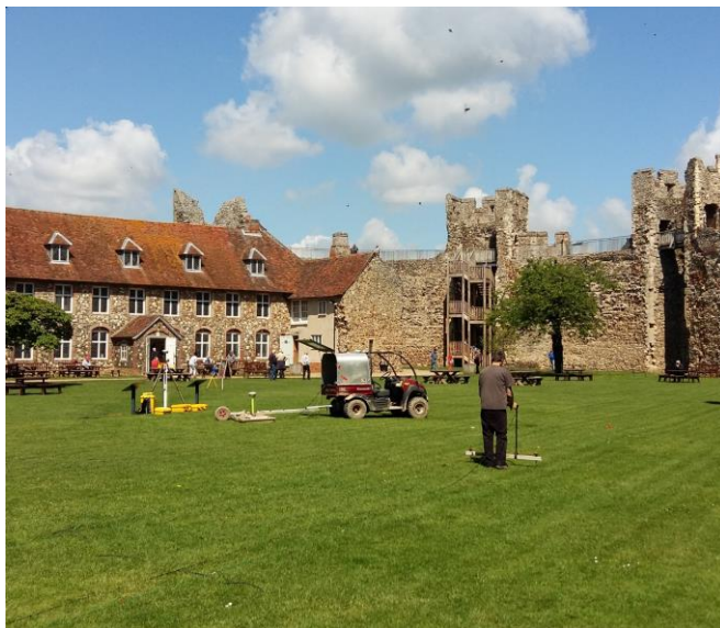
Figure 3: Earth resistance (shown right) and GPR survey were used to investigate the inner ward at Framlingham castle where the results confirmed the location of the former east cloister range.
