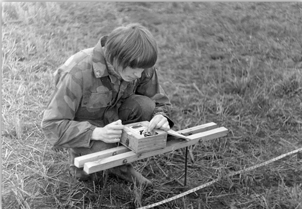
Figure 7: Chris Brooke: I've managed to dig out the pictuer of me, age 17, using a home-built 2-probe resistivity rig in 1975. No comfortable height, no logging, analogue meter, taped connections... In case you are wondering it worked perfectly and plotted the Roman road in Nottinghamshire I was seeking in textbook fashion. For those who knew him well this impressed Arnold Aspinall no end when it came to my interview at Bradford!
