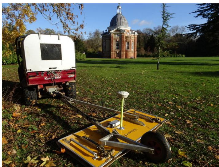
Figure 5: GPR survey at Wrest Park helped identify the location the buried plinth for the Duke of Kent’s monument, original gravel paths and two land drains.
