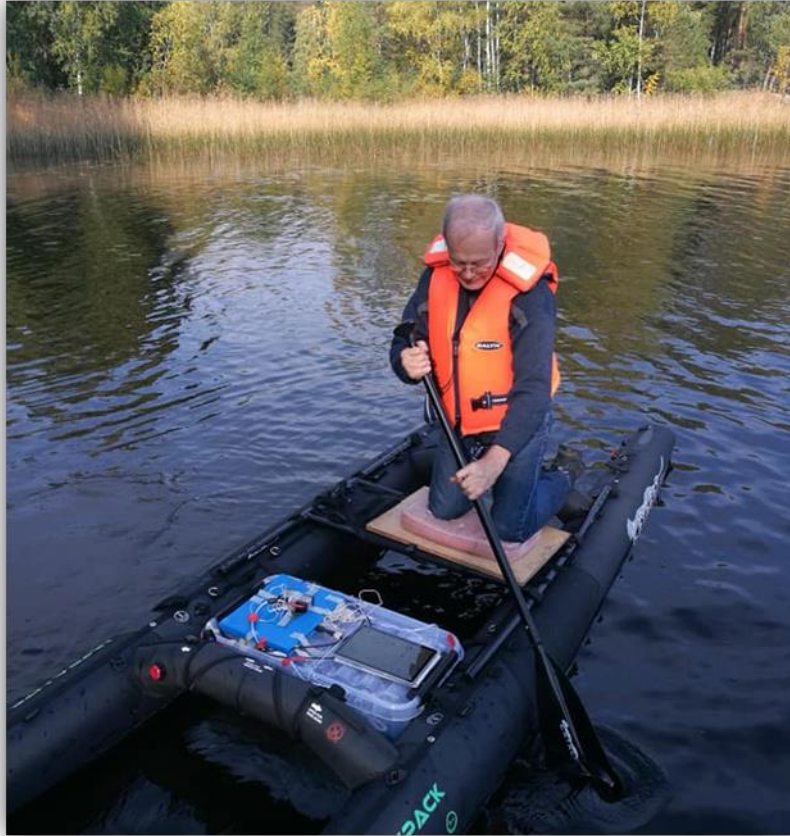
Figure 8: I am developing a new type of GPR antenna. It is in the plastic box in front of me in the float, called Kayacat. This time I was testing my GPR in the lake. I can also see the bottom at the same time and spot as the GPR. The picture was taken by Armi Temmes, my cousin. – Veli Voipio
