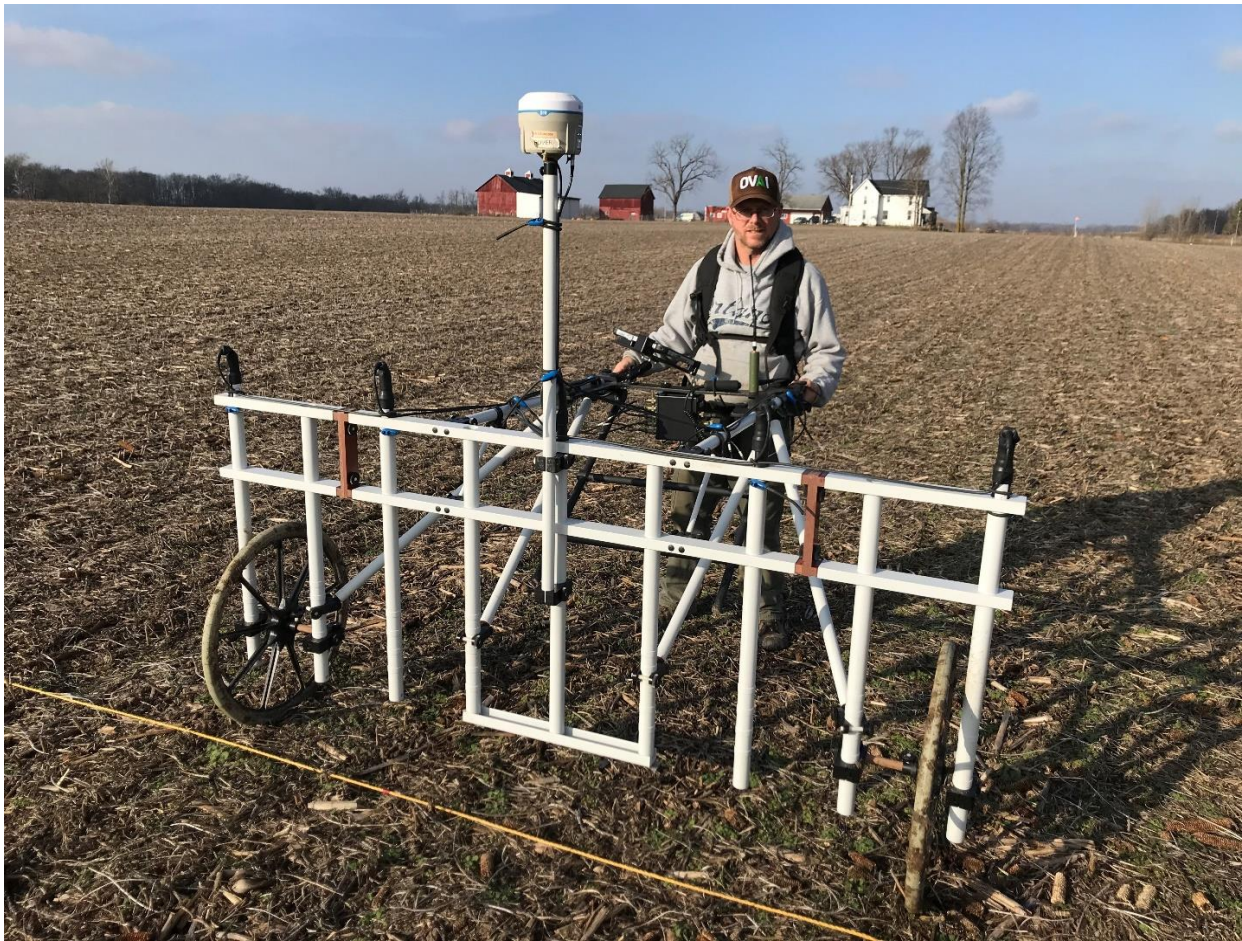
Figure 2. The Sensys MXPDA fluxgate gradiometer system used for the survey at Bertsch.
