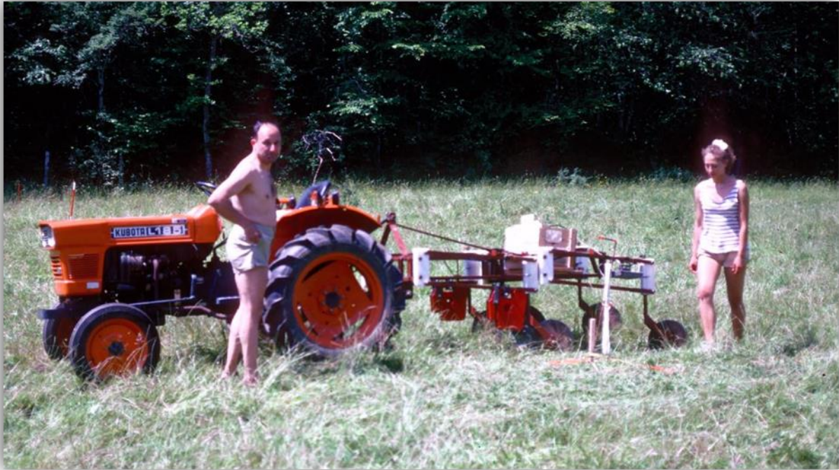
8. The Past. This picture from Michel Dabas proves that motorized systems are nothing new in archaeological prospection: In 1986 the team, including also Albert Hesse, Alain Tabbagh and Alain Jolivet, was testing the first automated system for resistivity mapping (RATEAU, now ARP) on the site of Minot-Brevon (France)
