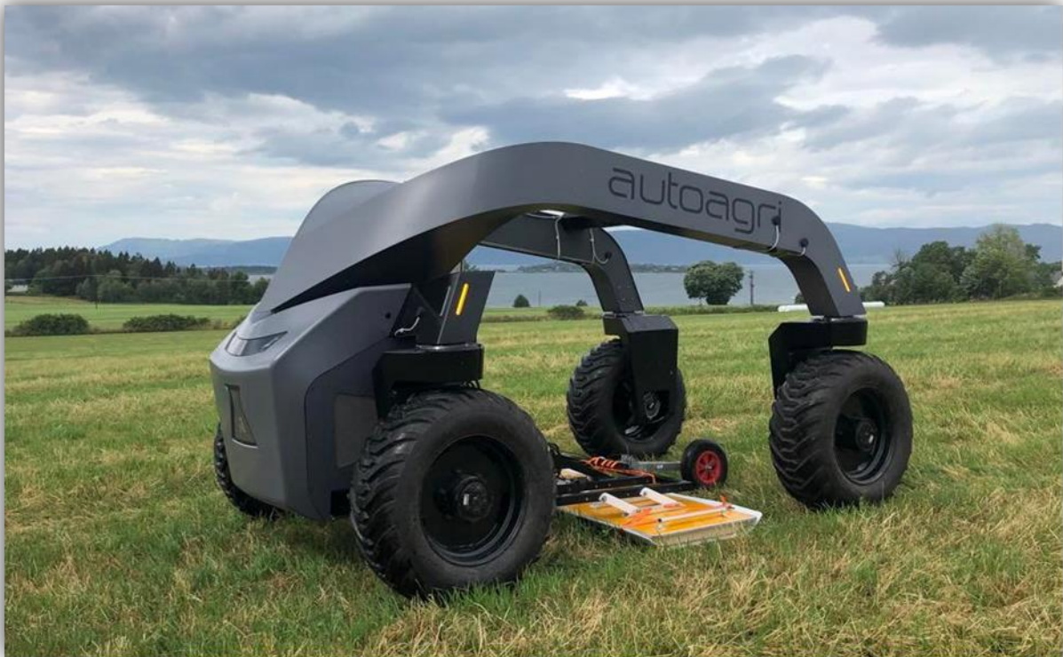
9. The Future. The picture of this amazing cyberpunk-like machine comes from Arne Anderson Stamnes: an autonomous cargo carrier. It can carry as much farming appliances as a 5-ton tractor, but weights just 2 tons!
