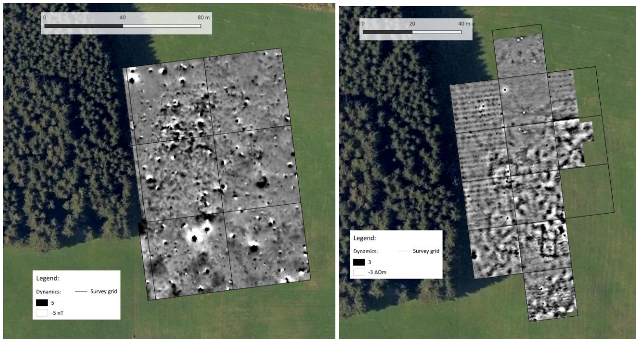
Figure 1: Magnetogram of the Roman villa rustica of Bertoldshofen surveyed in 2001. Caesium-Magnetometer Scintrex Smartmag SM4G-Special, Duo-Sensor-configuration, Dynamics \pm 5 nT in 256 greyscales, sampling rate 50 x 25 cm, interpolated to 25 x 25 cm, 40-m-grids. Archive-Nr. Ber01a (© Helmut Becker, Florian Becker & Roland Linck (BLfD); Digital orthophoto: Bayerische Vermessungsverwaltung).
