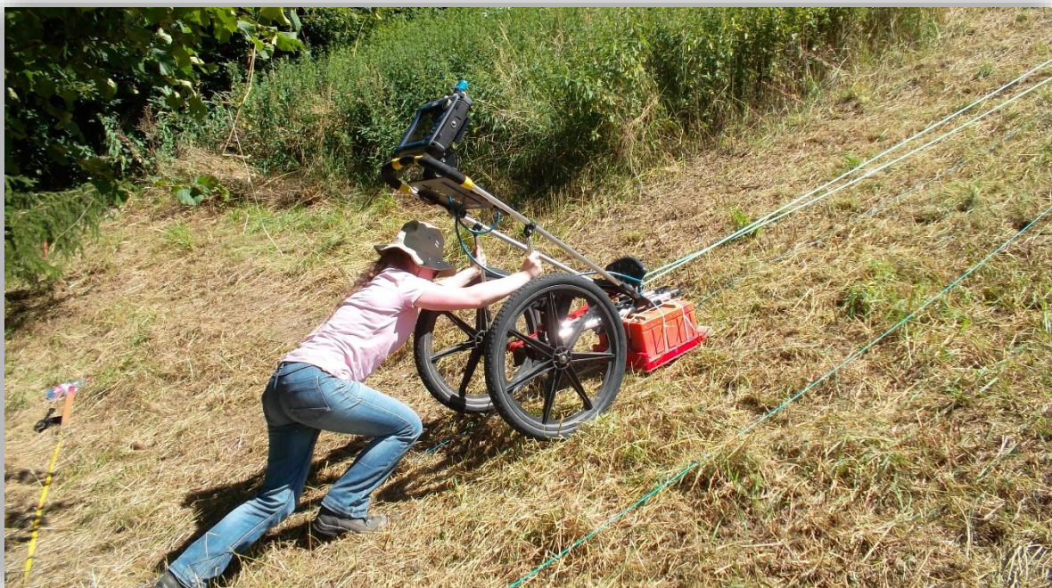
9. Crazy GPR survey at a 45° steep hill in a search of a possible Roman theatre in Southern Bavaria. The standard GPR equipment was modified to fit the special requirements of the survey area. The kit was pulled with a rope and a tackle from above. – Roland Linck
