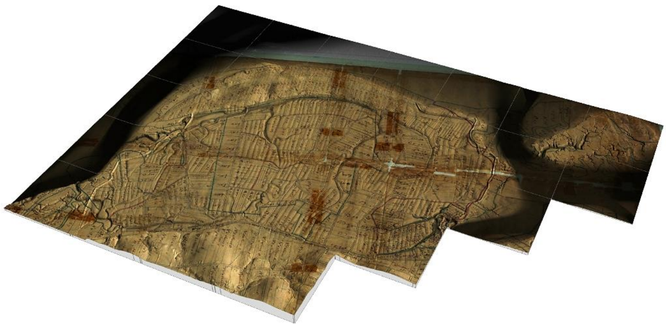
Figure 2: 1760s cadastral map of Grand-Pré georeferenced and applied to 2019 LiDAR-derived bare earth digital elevation model. Data courtesy of Province of Nova Scotia.
