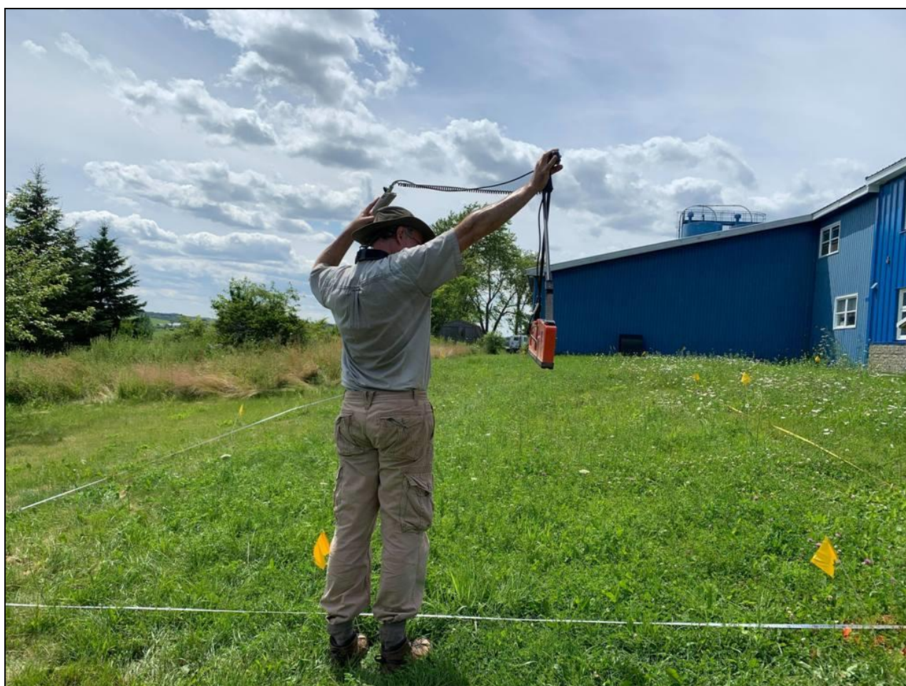
Figure 4: Raising the EM38B at the start and end of every survey line creates a ‘nose’ and ‘tail’ of zeroed readings on each line that can be used to help compensate for drift.
