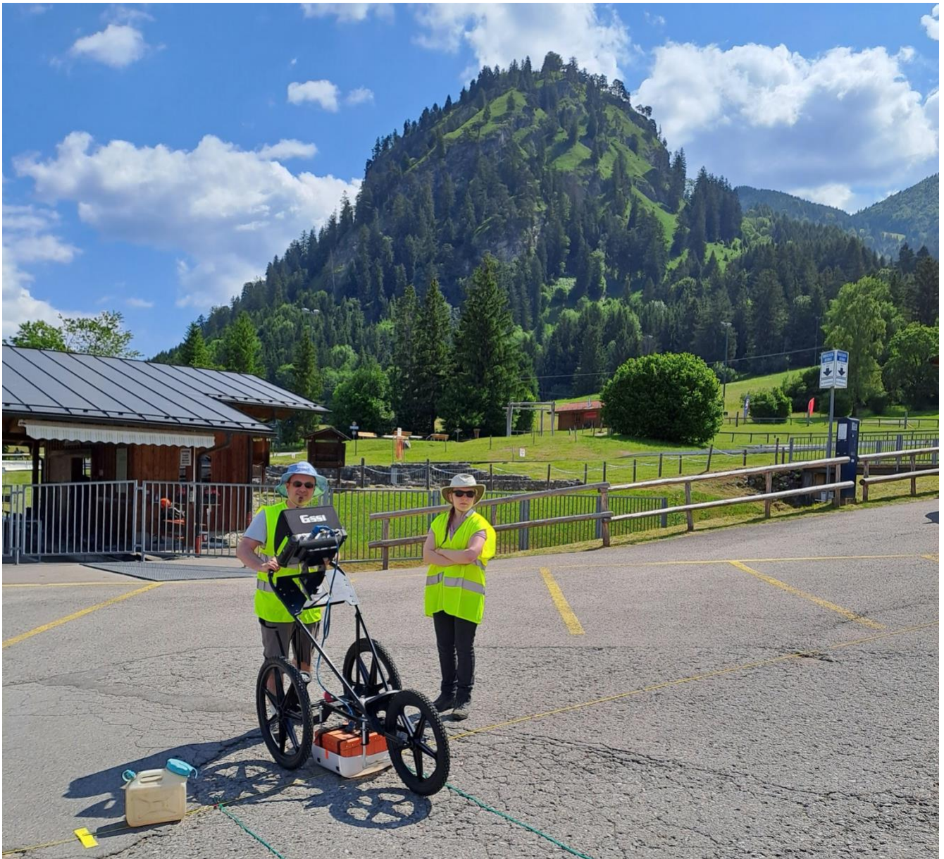
Figure 2: GSSI SIR-4000 radar system at the Roman site near the Tegelberg (Photo: Florian Becker, BLfD).
